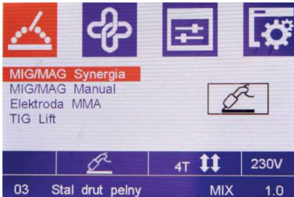
Figure 5: Choice of welding method (selected: MIG/MAG Synergia)
