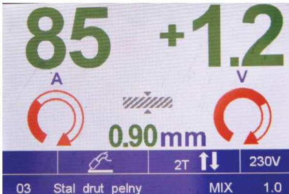
Figure 6: Welding parameter setting (program 03, intensity 85 A, arc length correction +1.2)
